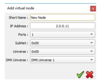
NB: With a fixture of several node, the Art-Net protocol uses consecutive universes for each of its ports. That is why it is needed to inform one universe only (the one which belongs to the device, same as for the SubNet). However, it is possible to send any software universe to each used port.
