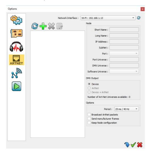
An Art-Net device is represented by a node which contains many ports, each port can receive 1 DMX universe. A simple Art-Net fixture shall be shown as a single port while an Art-Net convertor/ DMX with 4 DMX outputs for example shall be shown as a 4 ports.
